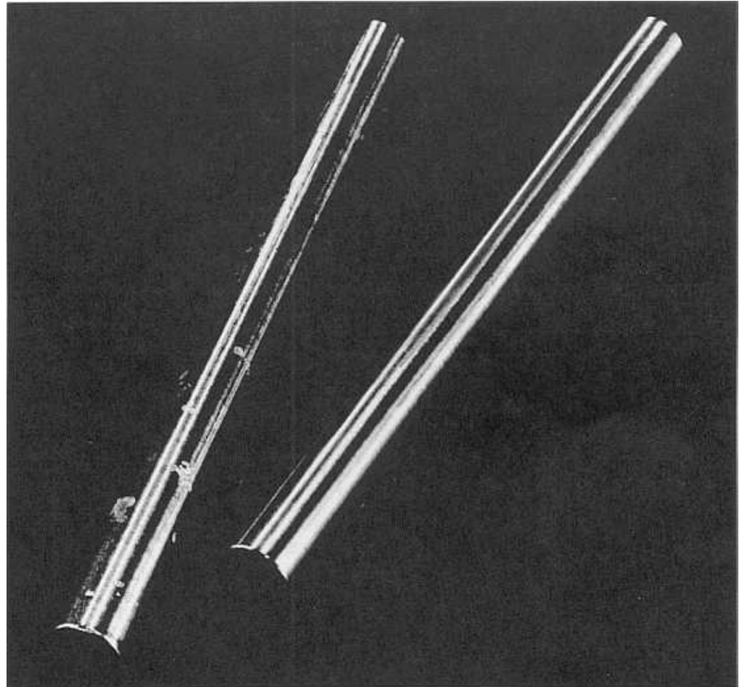
These two bars are immersed in quiet seawater for nine months. Bright shiny bar at right is ~~HP~~Alloys NITRONIC 50 stainless steel, and at left is Type 316 stainless steel showing considerable pitting and crevice corrosion.
